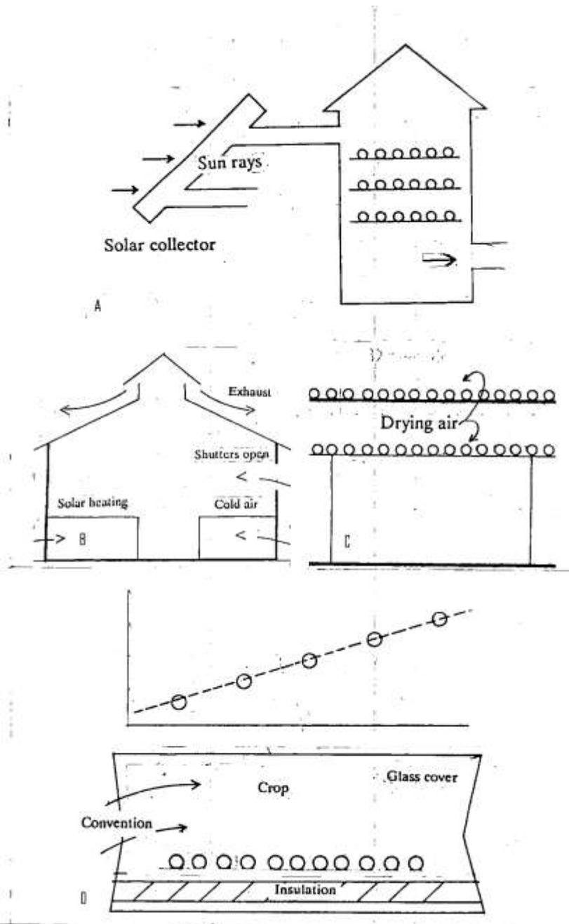
Fig. 1. Indirect dryer (A), Air circulating in the glass roof dryer for solar heating mode (B), Direct (Simple) and improved sun dryer (C) and mixed type solar dryer (D). Modified figure (Anwar *et al.*, 1991).
