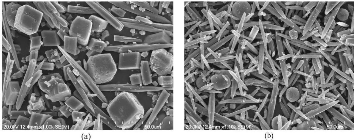
Fig. 2. (a) Scanning Electron Microscopy (SEM) image that shows the formation of calcite precipitate by *Bacillus sphaericus*. (b) SEM image that shows the formation of calcite precipitate by *Bacillus subtilis*. (Wiktor and Jonkers, 2011; Jonkers *et al.*, 2010).
