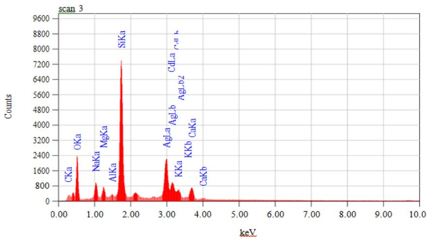
Fig. 3. EDS Spectrum of Silver Nanoparticles of Fungal Sample 5E
