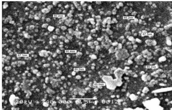
Fig. 2. SEM image of AgNPs using fungal sample 5E cell filtrate with radiation provision and salt concentration of 0.4M.
