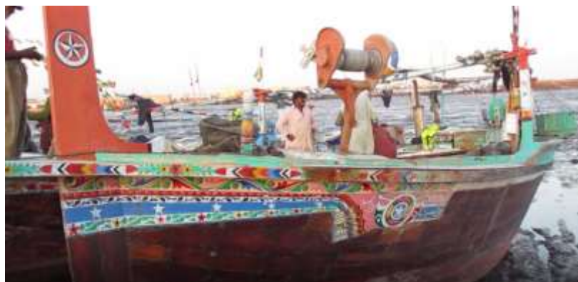
Fig. 2. A “hora” boat modified for operation of longline fishing. Installed line hauler is visible in the photo.
