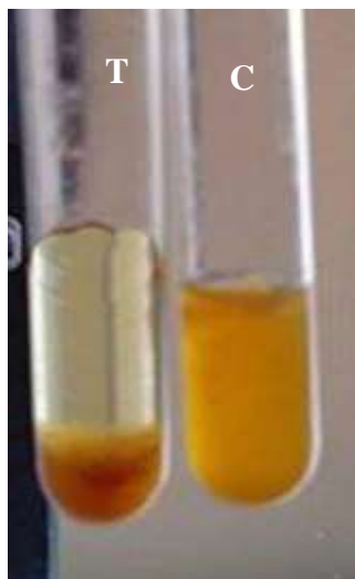
Fig. 9. Apple juice clarification after 24 h. Test tubes “C” and “T” representing “control” and “test” samples.
