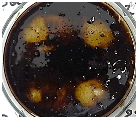
Fig. 1. oil spreading assay showing highly active biosurfactant producers, the changes seen in the oil present in the systems, compared to the control (water) without any change.
