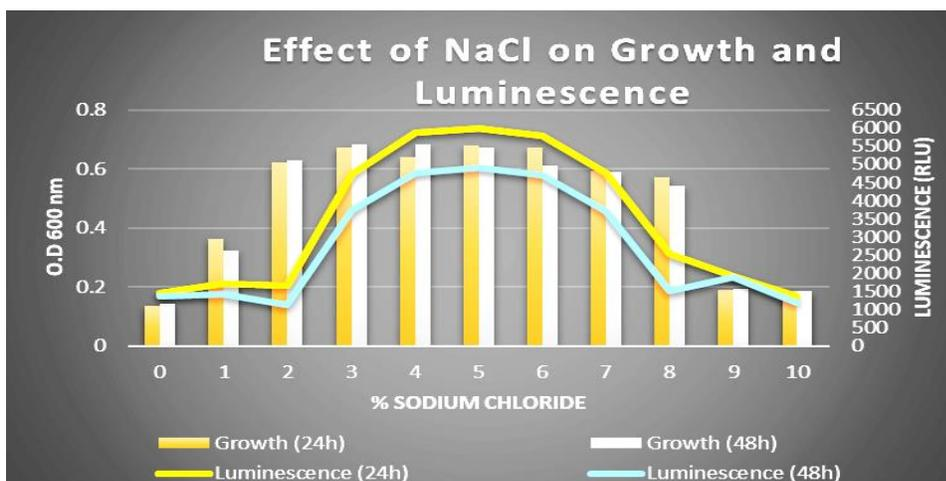
Fig. 4. Relationship of growth and luminescence in ASW supplemented with 1% glycerol, dosed with different concentration of NaCl.
