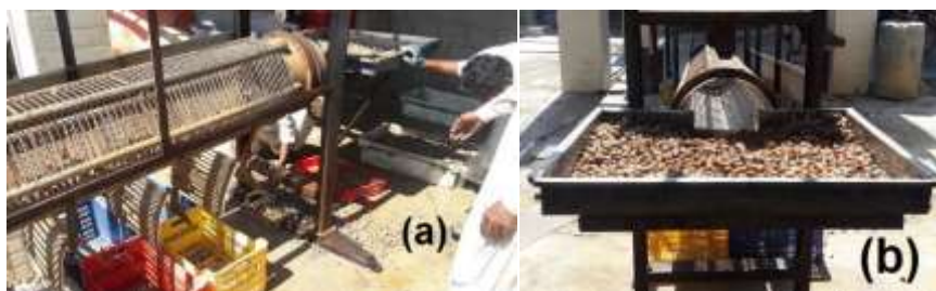
Fig. 6. (a) Locally designed machine which is used for grading of Babylonia spirata . (b) The largest preferred size is (50 to 80 pieces per kg) is accumulated in the last tray.
